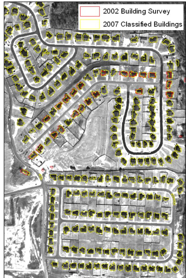
Figure 4. 2007 rooftop classification results obtained with the models developed using the 2003 image.
