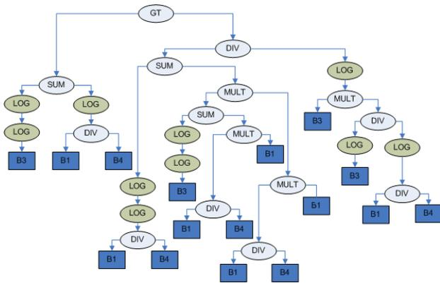
Figure 3. Example of non-linear model developed to spectrally separate asphalt-based materials from the remaining image background for QuickBird images.
