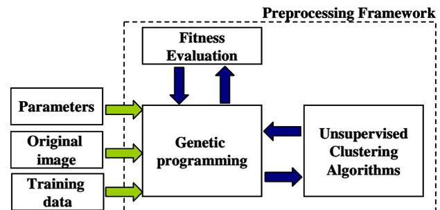
Figure 2. Conceptual diagram illustrating the main components of the evolutionary framework.
